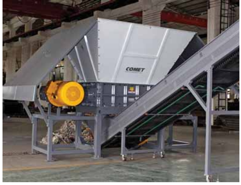
Feed to shredder hopper using conveyor, loader or forklift
